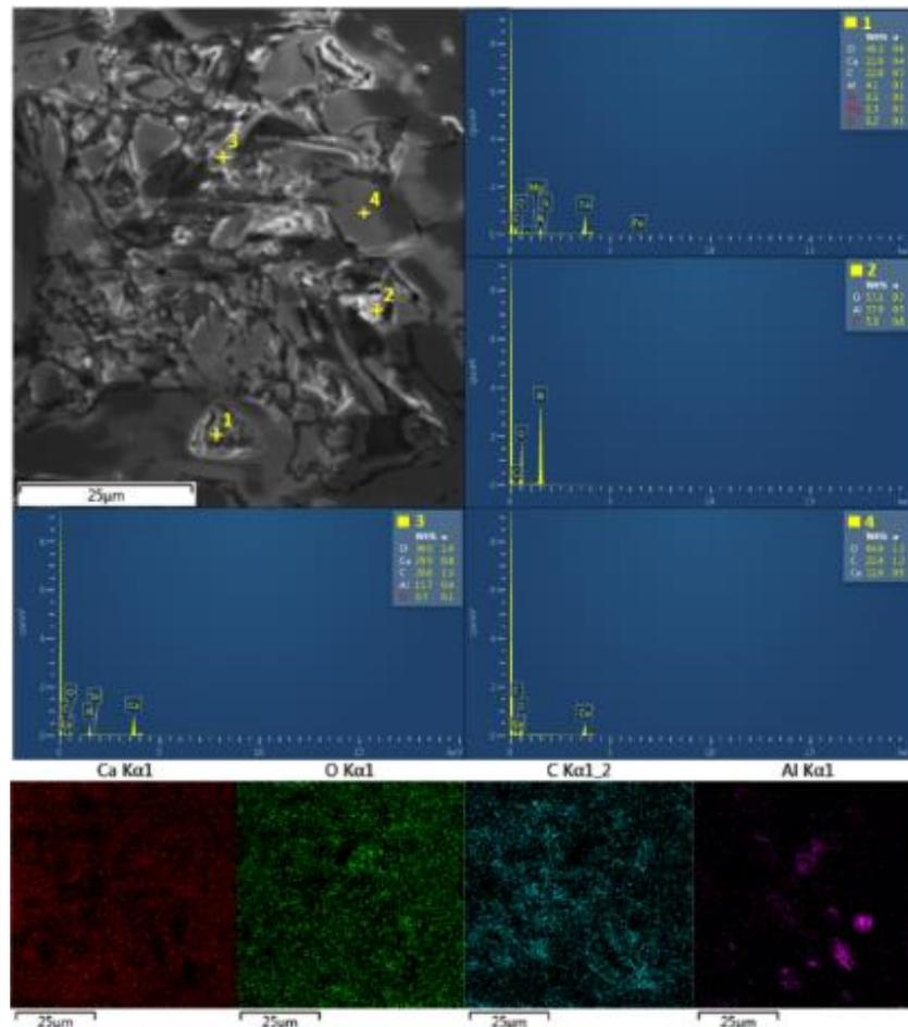
**Figure 9** - Microchemical maps of the P02 point with backscattered electron images of the elements Ca, O, C, and Al obtained by EDS probe. The colored areas show the presence of the chemical element highlighted in the center of each image. Oliveira et al. (2023).
